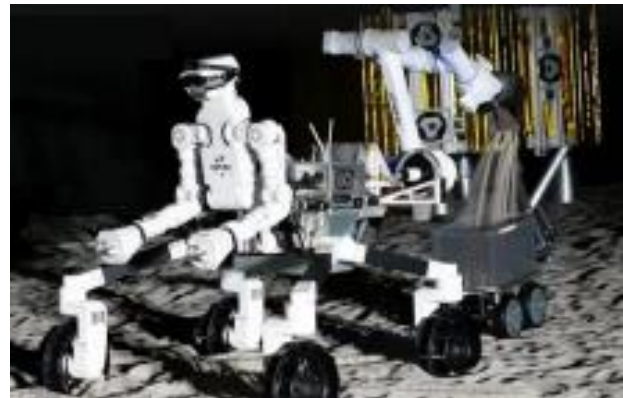
Fig. 2: GITAI Rover with a re-positionable arm, pouring sandy sample into a sample container.
