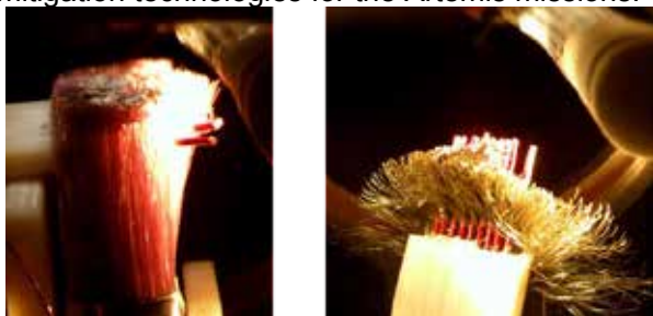
Figure 1: 3D-EDS experiments conducted by Shoot for the Moon for NASA’s 2021 BIG Idea Challenge. Experiments were conducted in vacuum with LHS-1 lunar simulant, copper wire and a nylon brush (left) and Thunderon® brush (right) Heating from a UV light caused the bristles to melt.
