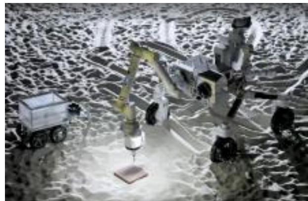
Fig. 3: Percussive sample fragmentation. All images are real demonstrations, not renderings.
