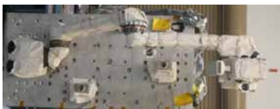
Figure 1: Blanketed SAMPLR Robotic Manipulator
