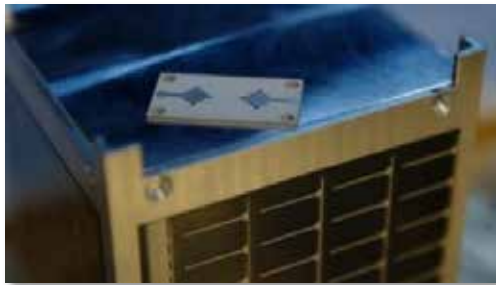
Figure 1. Lunasonde's miniaturized metamaterial-based antenna in relation to a 1U CubeSat.
