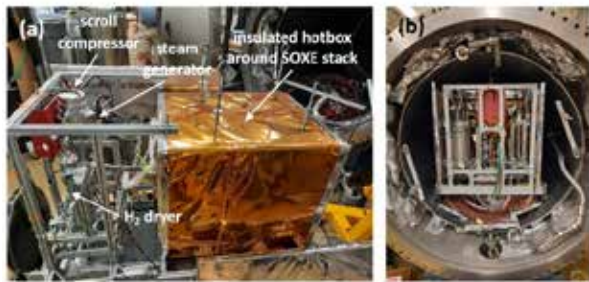
Fig. 1. a) Lab-scale electrolysis system. b) BOP and SOXE stack hotbox inserted into the vacuum chamber with the main door open before testing.
