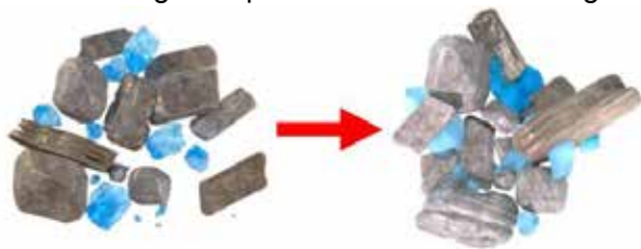
Figure 1: On the left, granular icy regolith is shown, and on the right PFG is shown as the result of granular icy regolith being pressed until the ice particles bond with the regolith particles and each other. Credit: Kevin Cannon
