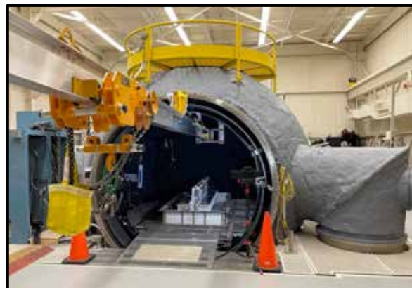
Fig 3- 15ft Thermal Vacuum Chamber with Spacesuit dust mitigation test equipment installed
