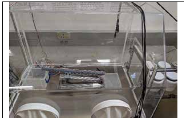
Fig. 3. The prototype of the electrostatic sieve as configured in a glove box ready to undergo testing of size separation of lunar simulants.
