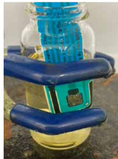
Figure 2: Generation of oxygen gas from lunar regolith digested in the ionic liquid EMI HSO 4 .
